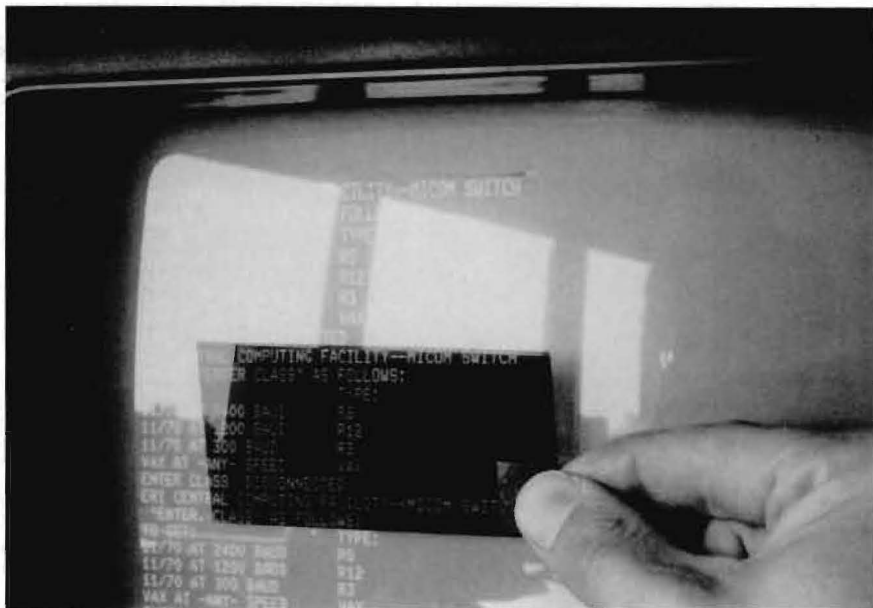
Figure 1: Control of reflections and glare from the VDT with circular polarizer.
